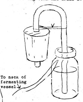
tubing. Bend over the top and retain with thread. Hang a small bottle of water on the end of the tube as illustrated.
