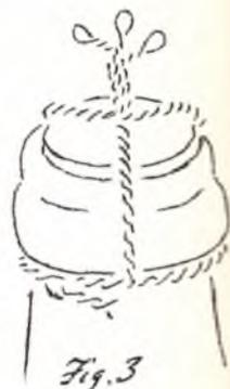
Use a soft supple wire for this, and start with a length of 22 inches. Bend and twist up as shown.
